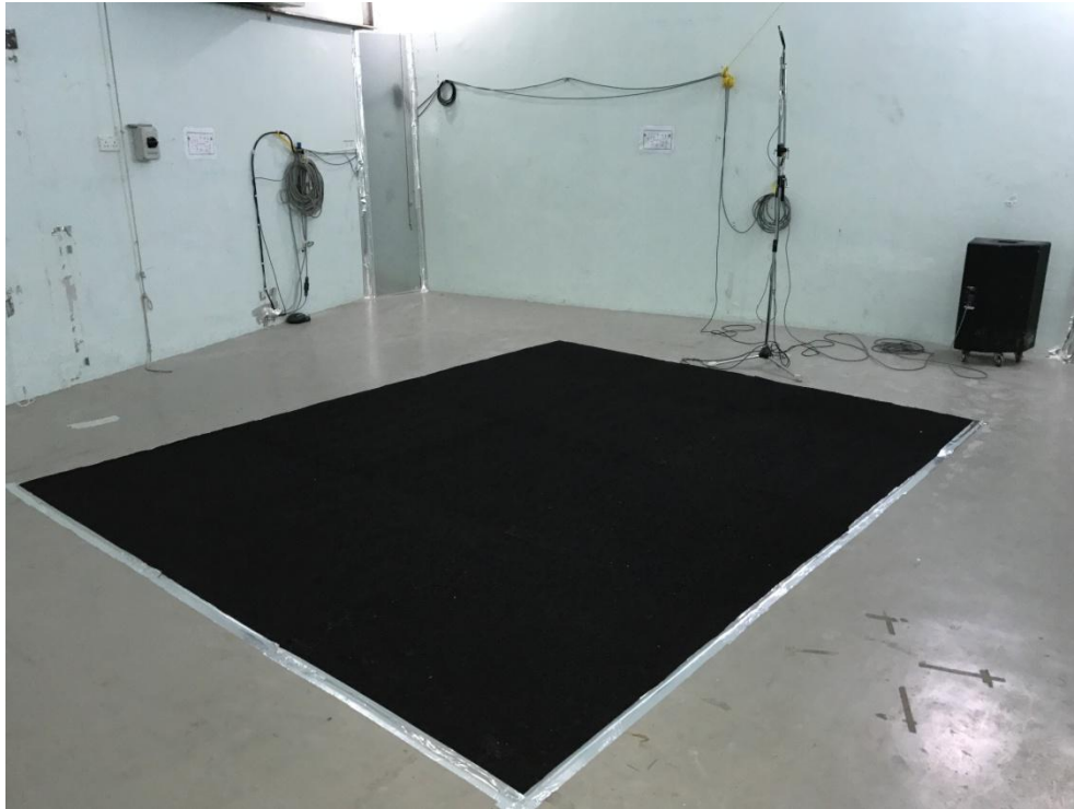
Figure 2 : 10mm thick Acoustec Sheet Nitrile Butadiene Rubber (NBR) laid on the floor as Type A mounting in reverberation room
